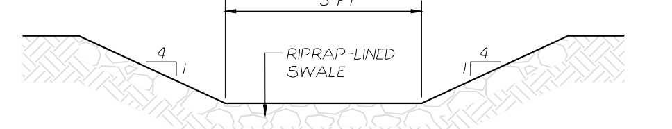
Overflow Swale Detail NOT TO SCALE
