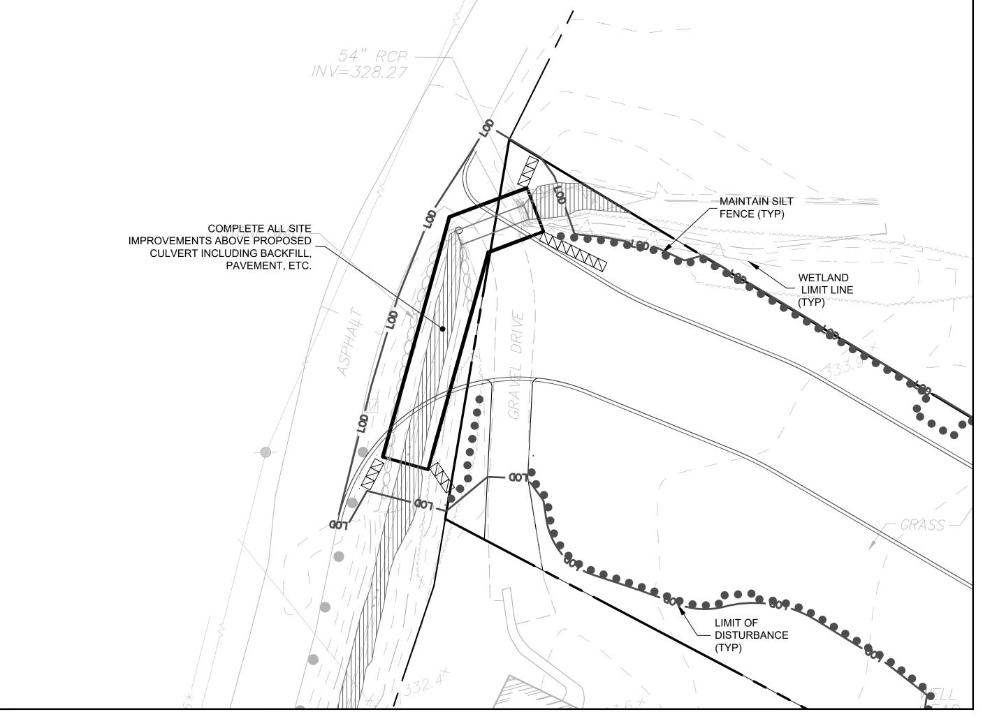
PHASE 2 - SOUTH SIDE FOOTING AND WINGWALL CONSTRUCTION
