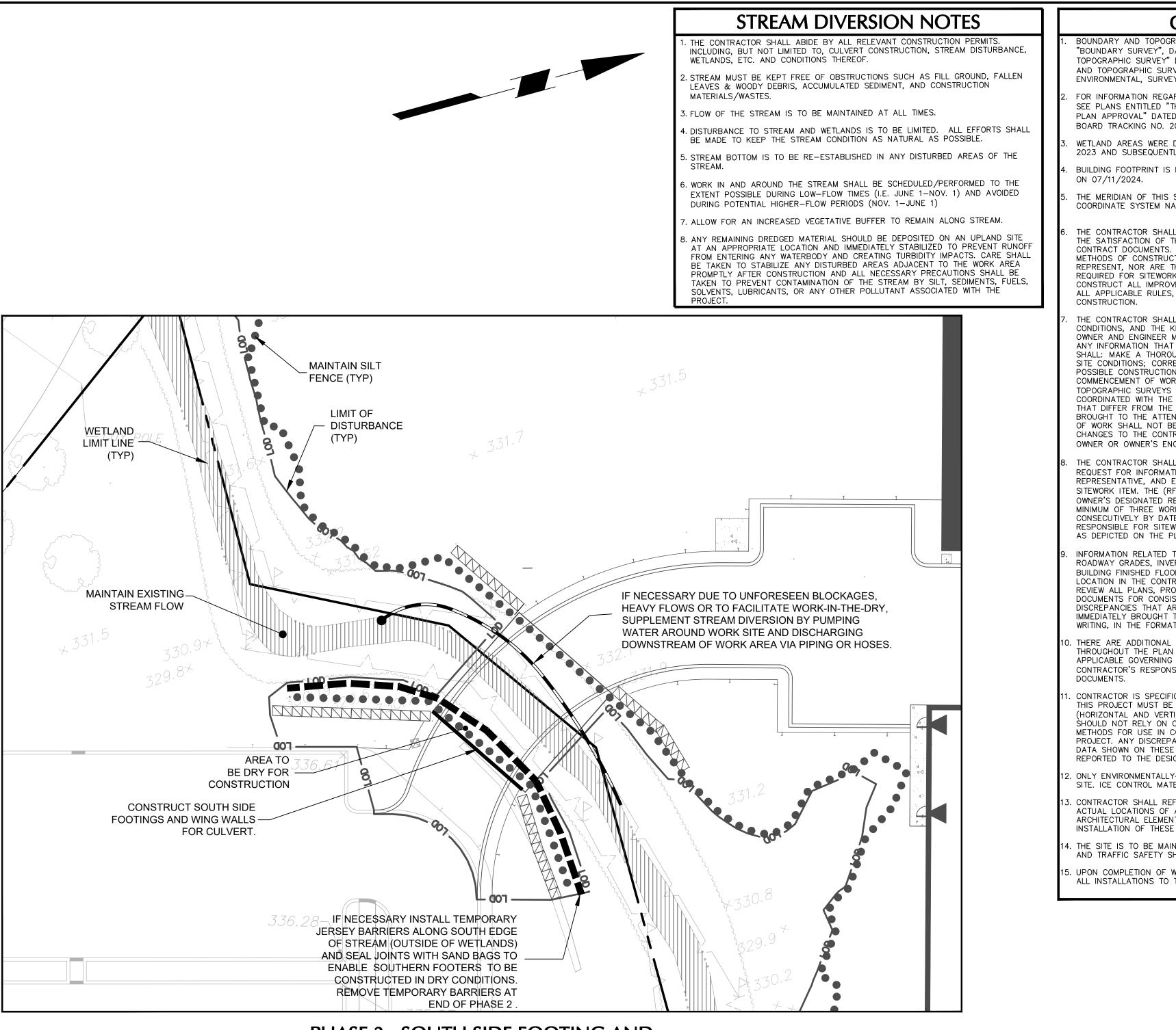
PHASE 2 - SOUTH SIDE FOOTING AND WINGWALL CONSTRUCTION
