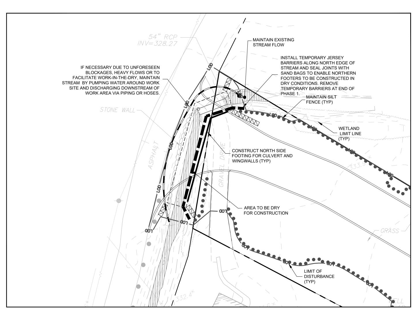
PHASE 1 - NORTH SIDE FOOTING AND WINGWALL CONSTRUCTION
