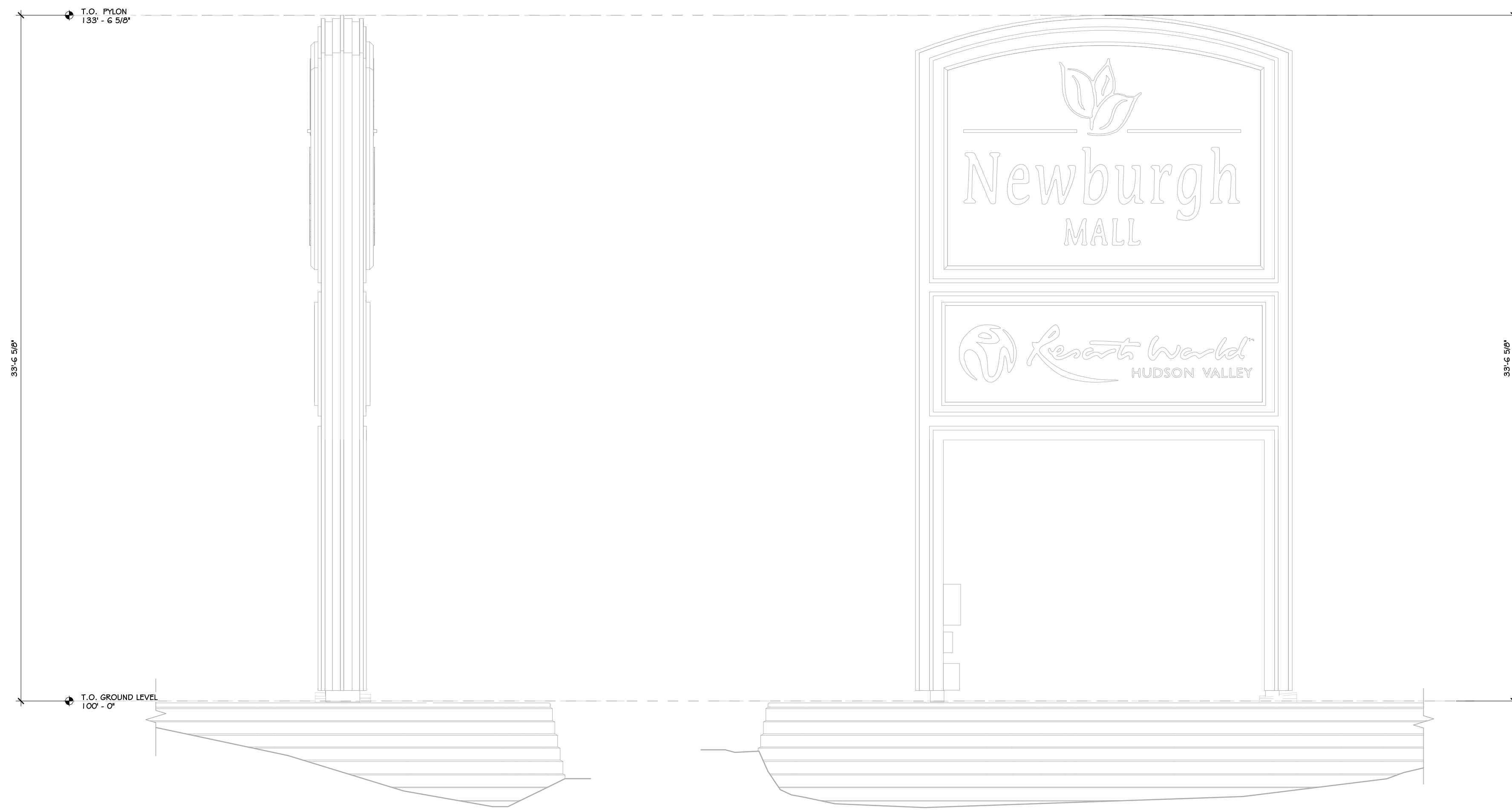
1 EXISTING DOUBLE SIDED MONUMENT SIGN PYLON DETAILS 1/4" = 1'-0"
