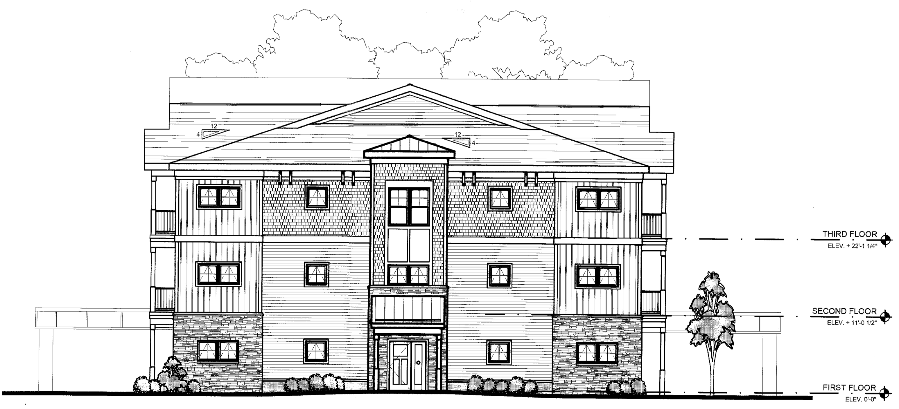
2 BUILDINGS 1 & 2: TYPICAL APARTMENT EAST / WEST ELEVATION SCALE: 1/8" = 1'-0"
