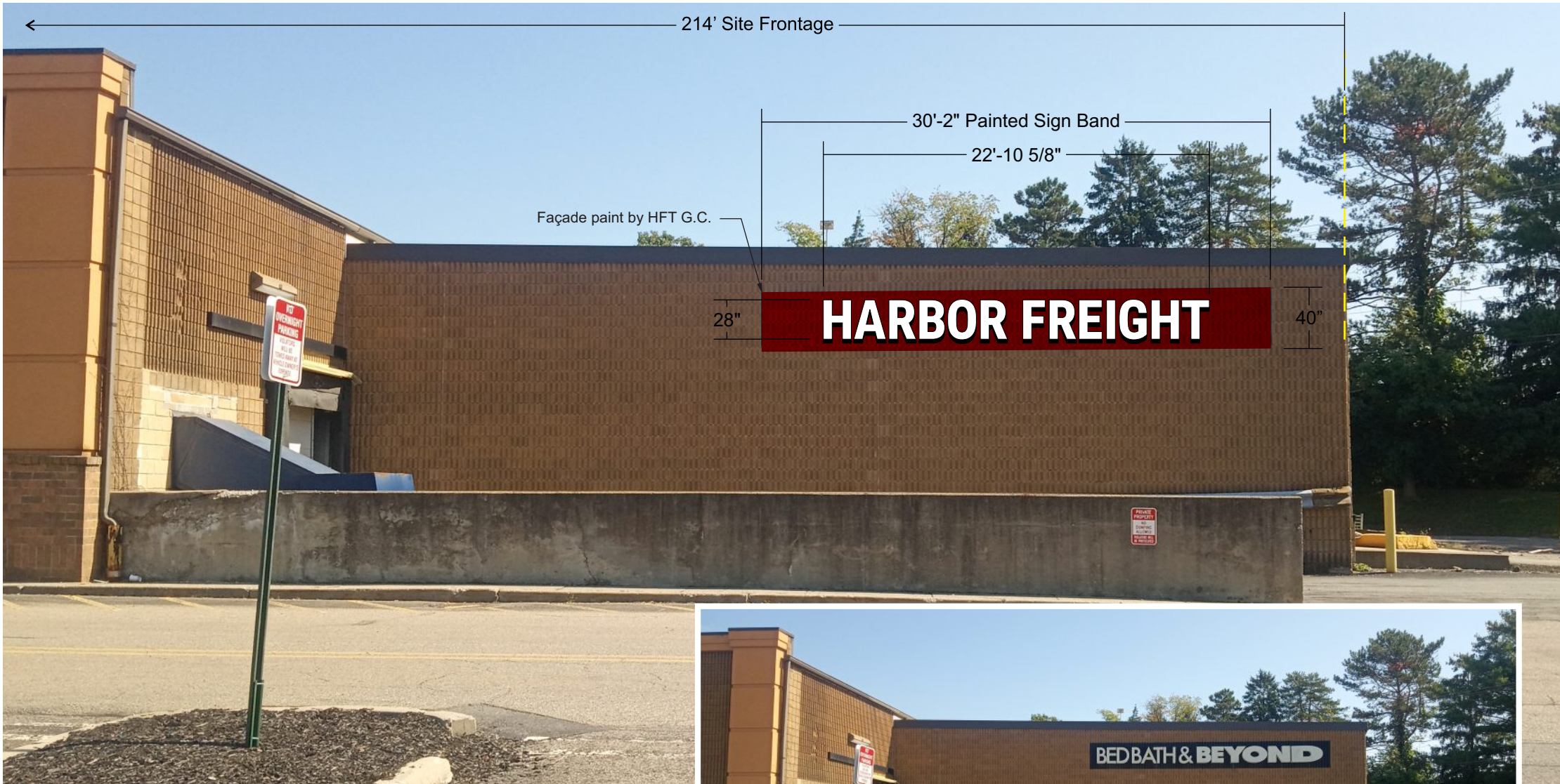
SIDE ELEVATION - Sign Type (B) (QTY:1) Channel Letters - Mounted To Wall Scale: 1/8" = 1'-0" = 1' (53.40 SQ FT)
