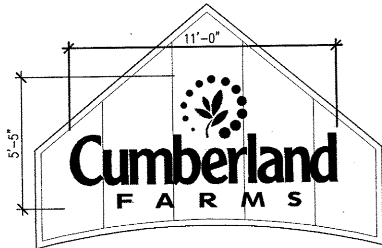
4 FRONT WALL SIGNAGE DETAIL A3.1 SCALE: 1/4"=1'-0"
