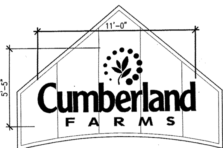
4 FRONT WALL SIGNAGE DETAIL A3.1 SCALE: 1/4" = 1'-0"
