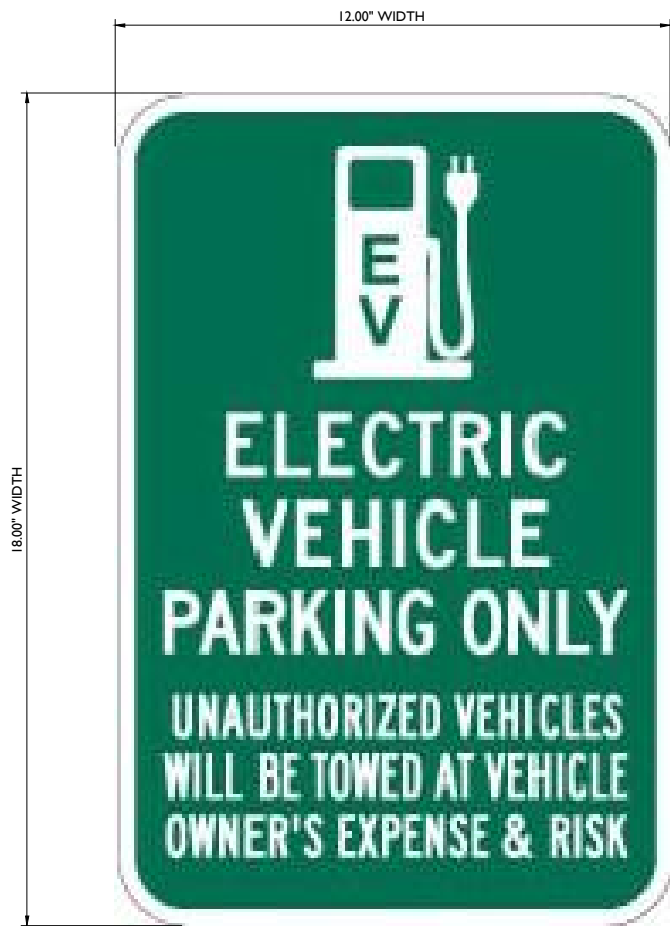
PARKING SIGN DETAIL NOT TO SCALE
