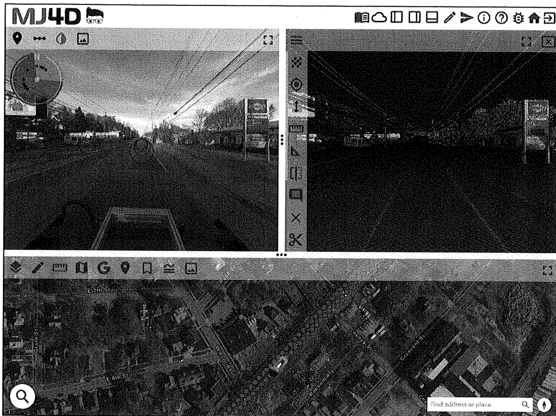
Figure 2: MJ4D displaying a mobile LiDAR collection
