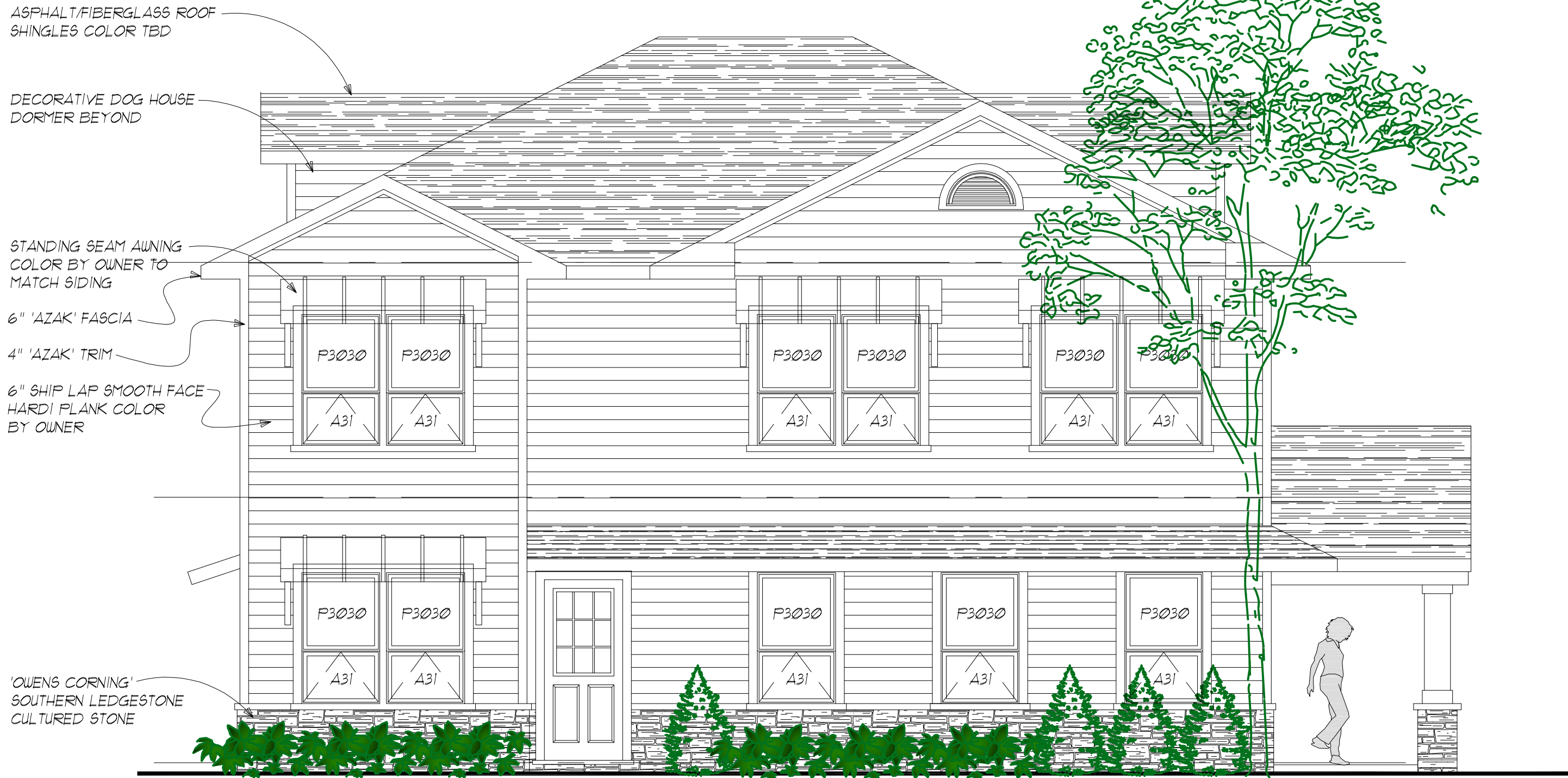
3 Proposed Front Elevation A-300 SCALE: 1/4"=1'-0"
